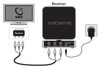
Fig. Connection example for Receiver
